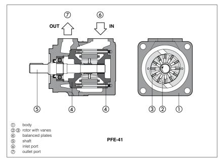
PFE are fixed displacement-twelvevane pumps, (2) (3) cartridge design with integral hydraulic balancing 4 for high pressure operation and long service life with low noise level.
