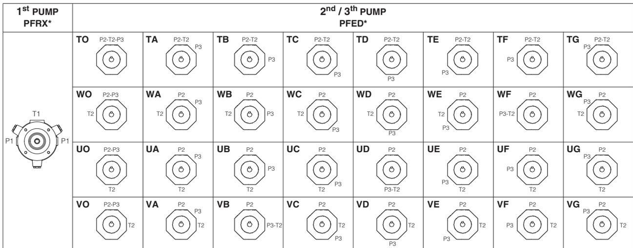
P1 outlet port of first element; P2 outlet port of second element; P3 outlet port of third element; T1 inlet port of first element; T2 inlet port of second element
