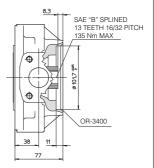
Drawing shows pumps with clockwise rotation (option D): pumps with counterclockwise rotation (option S) will have inlet and outlet ports inverted
