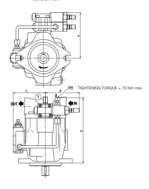
① = Regulation screw for max displacement. Adjustable range 50% to 100% of max displacement). In case of double pump the regulation screw is not always available, please contact our technical office.
