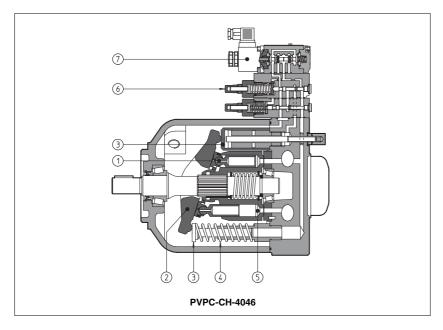
PVPC are variable displacement axial piston pumps for high pressure operation, with low noise level, suitable for hydraulic oils or synthetic fluids having symilar lubricating characteristics.
