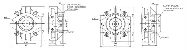
Drawing shows pumps with clockwise rotation (option D): pumps with counterclockwise rotation (option S) will have inlet and outlet ports inverted
